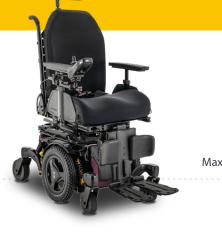
Powered Seat Lift Powered Tilt Powered Recline Q-Logic 3e Control System 2 x 62 ah Batteries 4 Mph (6 Km/h) Motors Max User Weight: 21 st 6lbs. (136 kg)
