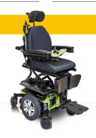
2" x 6" Flat Free Rear Castors ATX Suspension System **NE+ Control System** 2 x 62 ah Batteries 4 Mph (6 Km/h) Motors Max User Weight: 21 st 6lbs. (136 kg)
