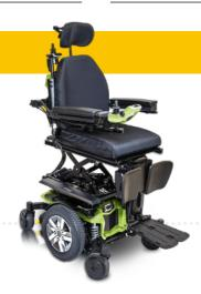
2" x 6" Flat Free Rear Castors ATX Suspension System **NE+ Control System** 2 x 62 ah Batteries 4 Mph (6 Km/h) Motors Max User Weight: 21 st 6lbs. (136 kg)
