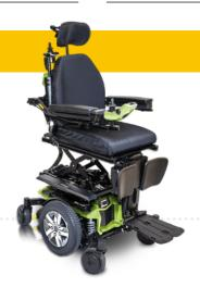
2" x 8" Flat Free Rear Castors ATX Suspension System **NE+ Control System** 2 x 62 ah Batteries 4 Mph (6 Km/h) Motors Max User Weight: 21 st 6lbs. (136 kg)
