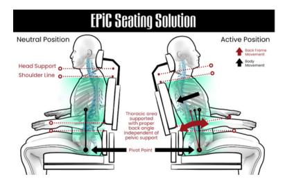
The postural management system incorporates an angle/height adjustable stationary pelvic support with a moveable thoracic back support. The system also incorporates an anatomical pivot point which helps to support movement without changes in the postural support devices.
