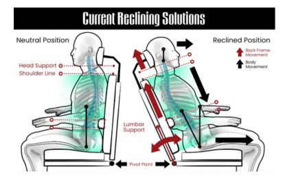
When the back support reclines, the back slides upward relative to the client's body causing friction and shear forces. As the back support returns to neutral position, sliding occurs at the pelvis creating friction and shear forces at the seat surface. Secondary positioning supports such as headrest and laterals also move in conjunction with the back support during recline, which will require mechanical readjustment by a caregiver.
